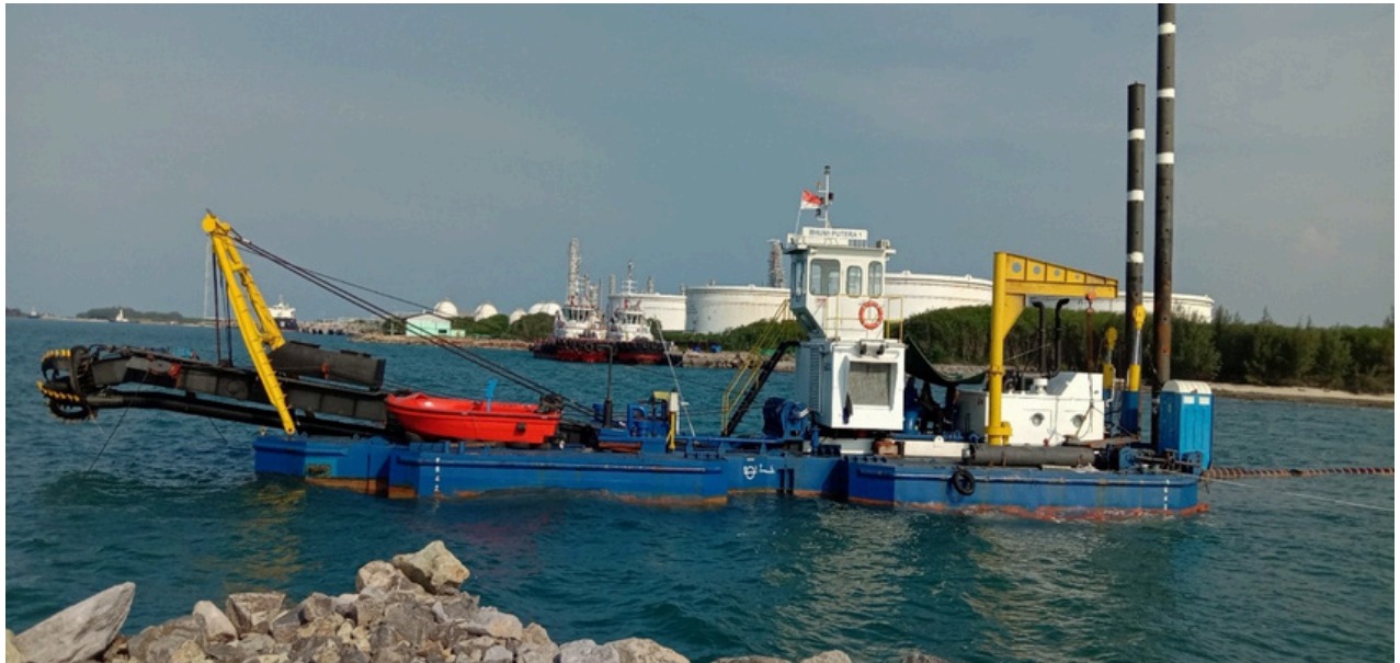
Cutter Suction Dredger
